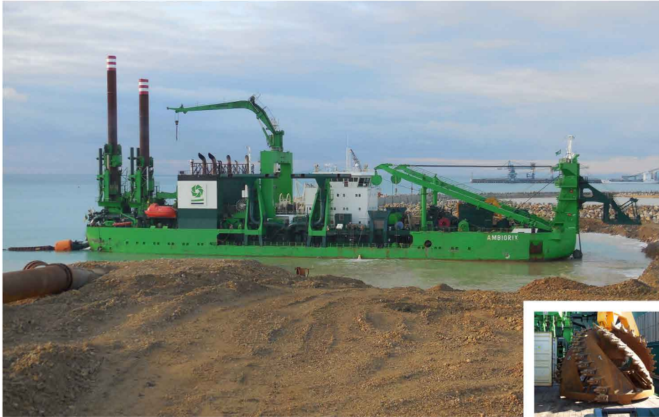
CUTTER SUCTION DREDGER AMBIOREX WITH A SPECIFIC ROCK CUTTER
